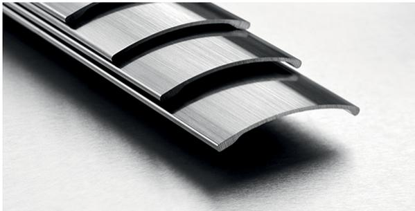
Rolex uses 904L stainless steel for its steel watch cases. 904L is mainly used in the high technology, aerospace and chemical industries, where maximum resistance to corrosion is essential. A superalloy, 904L is extremely resistant and highly polishable. It maintains its beauty even in the harshest environments. 904L steel also provides a perfect complement to the precious metals used by Rolex.
